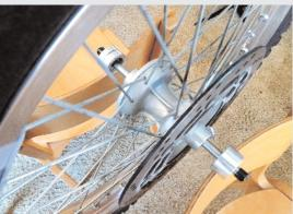
The large stands that use a pair of knife edge bearings on each side to support standard axles have the problem that their bearings are fully exposed to frictioninducing dirt and corrosion, and since you're using your own axle, you can't be sure it's smooth or straight enough for perfect accuracy. Also, these stands take up a lot of space, which is always at a premium in a home garage.
